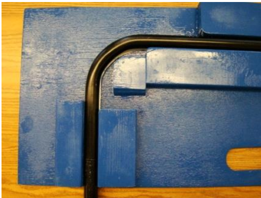
Fig. 13.13. Portion of template for shaping the bed rail. The rail is shown in black.
