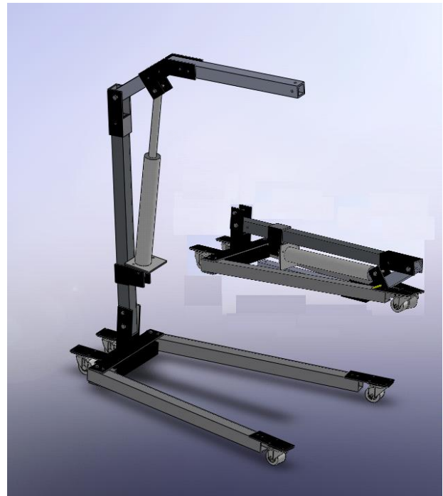
Fig. 13.14. Computer rendering of the collapsible hoist frame in both its stowed and deployed configurations.
