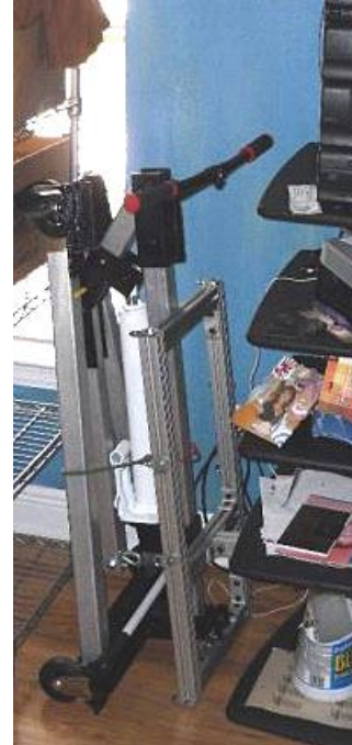
Fig. 13.15. Hoist with cradle in its folded or travel configuration.
