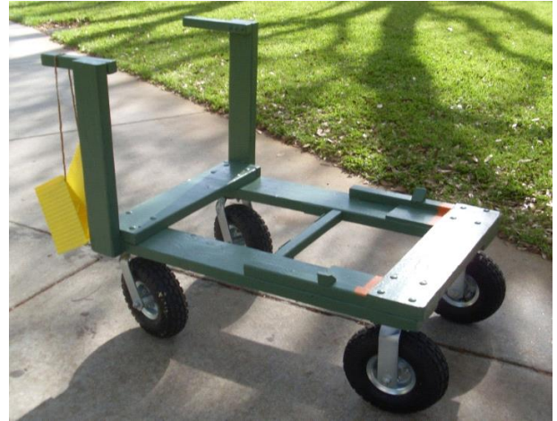
Fig. 13.8. Wheeled base with chocks in storage position.
